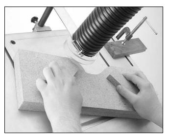
Figure 27. Work is supported by the guide bearing.
